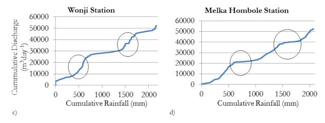
Figure 5-4: Double mass curve of cumulative observed discharge vs. satellite rainfall
