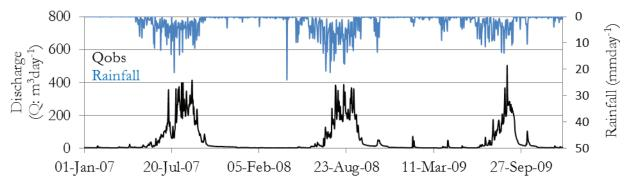
Figure 5-5: Observed stream flow at Melka Hombole station used for calibration and validation of the model
