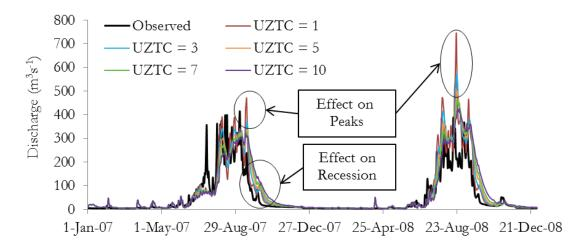
Figure 5-9: Sensitivity of the model to changes in the Upper Zone Time Constant parameter
