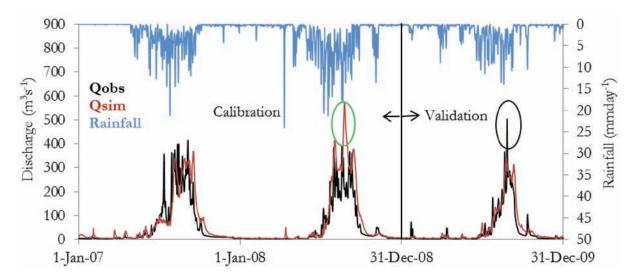
Figure 5-12: Simulated and Observed hydrograph for the period 2007 – 2009 at Melka Hombole gauge station
