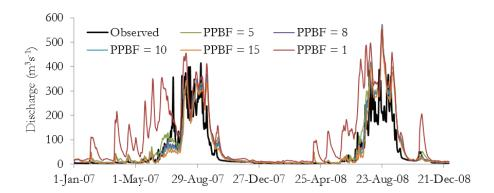
Figure 5-10: Sensitivity of the model to changes in the Power Preferential Bypass Flow parameter
