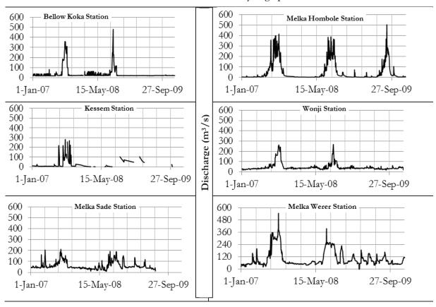
Figure 3-4: Observed stream flow hydrograph of selected 6 stations
