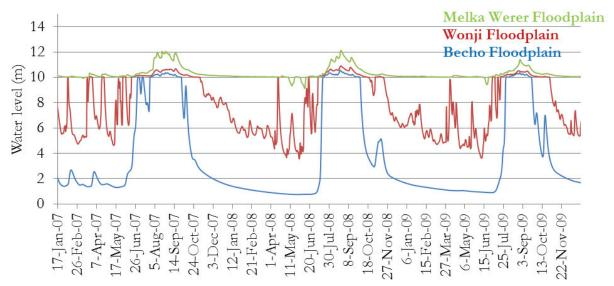
Figure 5-14: Water level simulation at the flood prone areas
