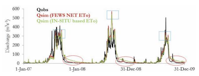
Figure 5-13: Comparison between observed and simulated hydrograph using FEWS NET and in-situ based ETo
