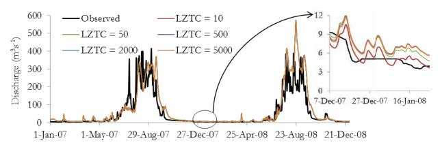
Figure 5-7: Sensitivity of the model to change in Lower Zone Time Constant parameter
