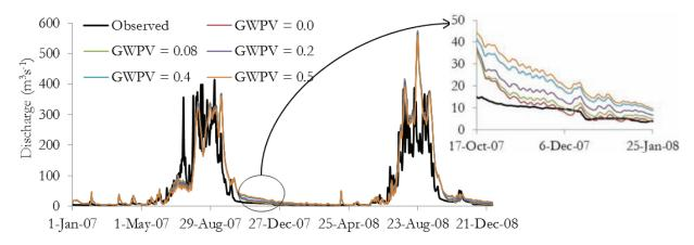
Figure 5-8: Sensitivity of the model to changes in the Groundwater Percolation Value parameter
