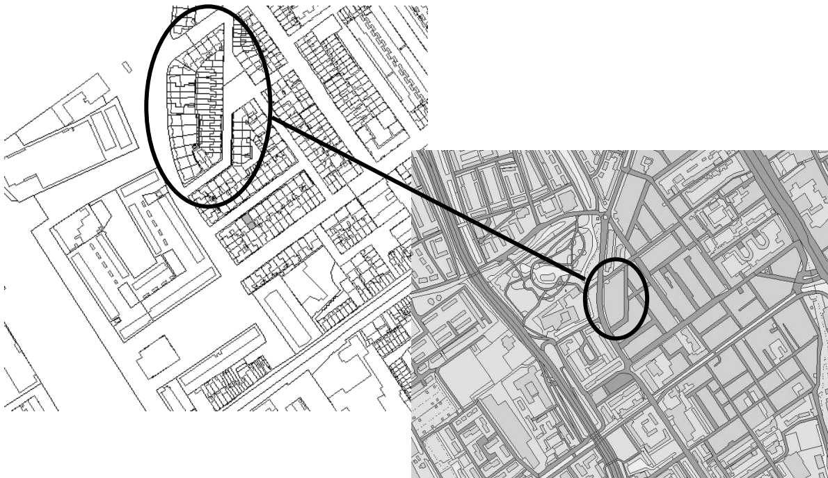
Figure 3: Using buildings from the Large Scale Map in the TOP10vec requires generalisation of the objects.
