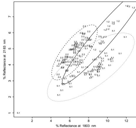
Figure 9.5: The scatterplots of two bands (1803 nm and 2183 nm) of three vegetation types with their 95% confidence ellipses make a fan-shape.
