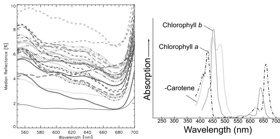
Figure 9.2: Median reflectance curves of 27 saltmarsh vegetation types in the visible part of the spectrum from 550 nm to 700 nm (a), and the absorption curves of plant pigments (b) (source: Purves et al. (1998)).
